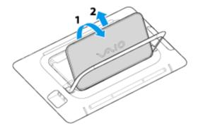
5. Slide the battery LOCK switch (1) to the unlock position.
